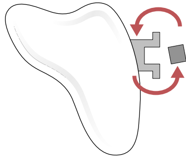
Figure 5.9 Placement of torsion or torque into the wire will counter the effect of tipping during bodily retraction.
